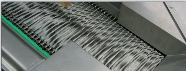
Stainless steel link band. Robust and temperature resistant
