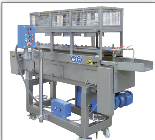
Variants: Water mist (pneumatic liquid spray diffuser) and air flow cooling (speed-controlled fans) with dust filtering
