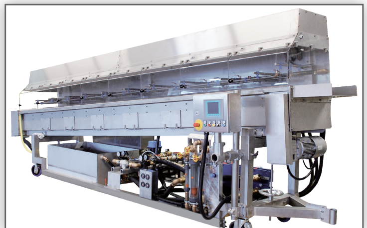
Variants: Water mist (pneumatic liquid spray diffuser) and air flow cooling (speed-controlled fans) – with integrated process water system, housing and comfort operation panel
