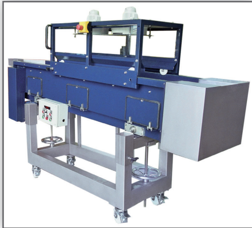
Variants: Air flow cooling (speed-controlled fans)
