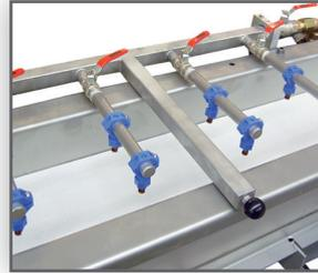
Easy-to-replace process water spray nozzles
