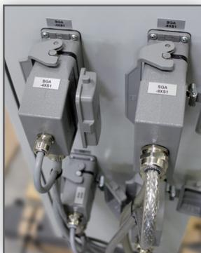
Interface for connecting a process data system
