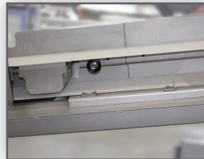
Quick, tool-free access to the strand conveyor belt for maintenance and cleaning
