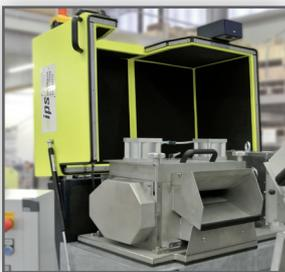
Easy access to the cutting head for cleaning or maintenance work
