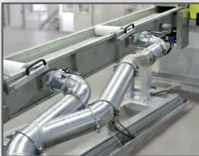
Integrated strand dewatering through the strand conveyor belt
