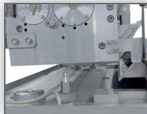
Quick-change cutting head with quick disconnection of the drives and pneumatics
