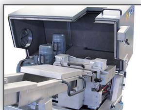
Very low noise level thanks to joint sound cover for drive and cutting head
