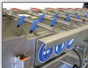
Specific cooling of the polymer strands before cutting
