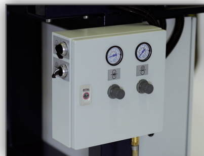
Standard: Pneumatic pressure on the upper feed roller
