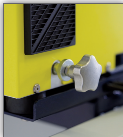
Standard: Adjustment of the feed roller gap during operation
