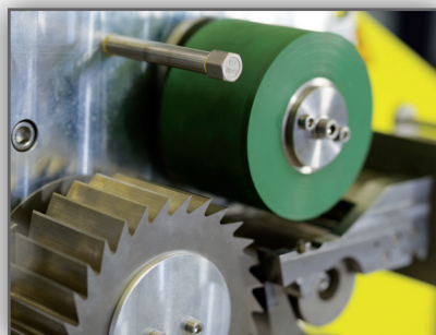
Cutting area cooling using compressed air
